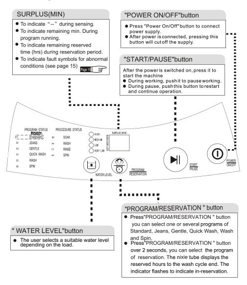
Remarks: 1. After pressing "POWER ON/OFF" to connect power supply, if the washing machine lasts idle more than 5 min, it would automatically shut off the supply.
